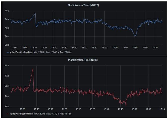
Fig. 4. Plasticization time of NB90 and NB220 machines.
