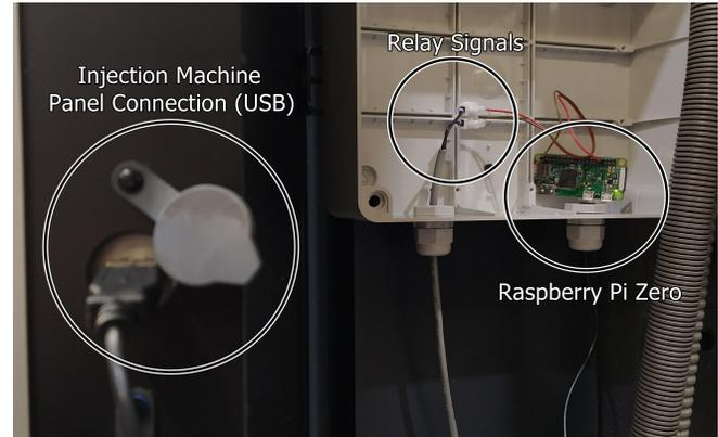
Fig. 2. Real system connected to the injection machine.
