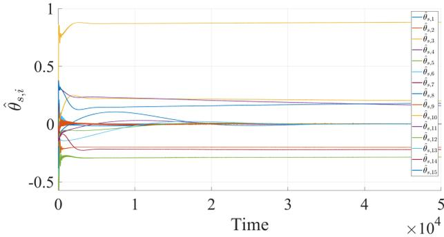
Fig. 1. parameter-estimation evolution through the standard adaptive observer. No sensor noise is considered  $\mathbf{v} = 0$
