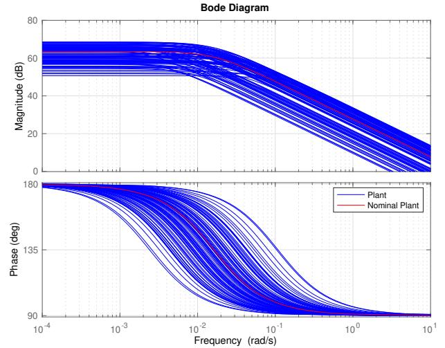
Fig. 2. Bode Diagram for different linear plants in the operational range.
