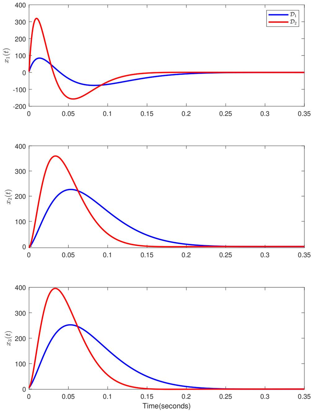
**Figure 4.** The closed-loop response by pole clustering in  $\mathcal{D}_1$  (blue) and  $\mathcal{D}_2$  (red).
