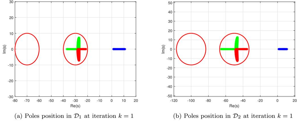
**Figure 2.** Position of the closed-loop frozen poles after the first iteration  $k = 1$ .
