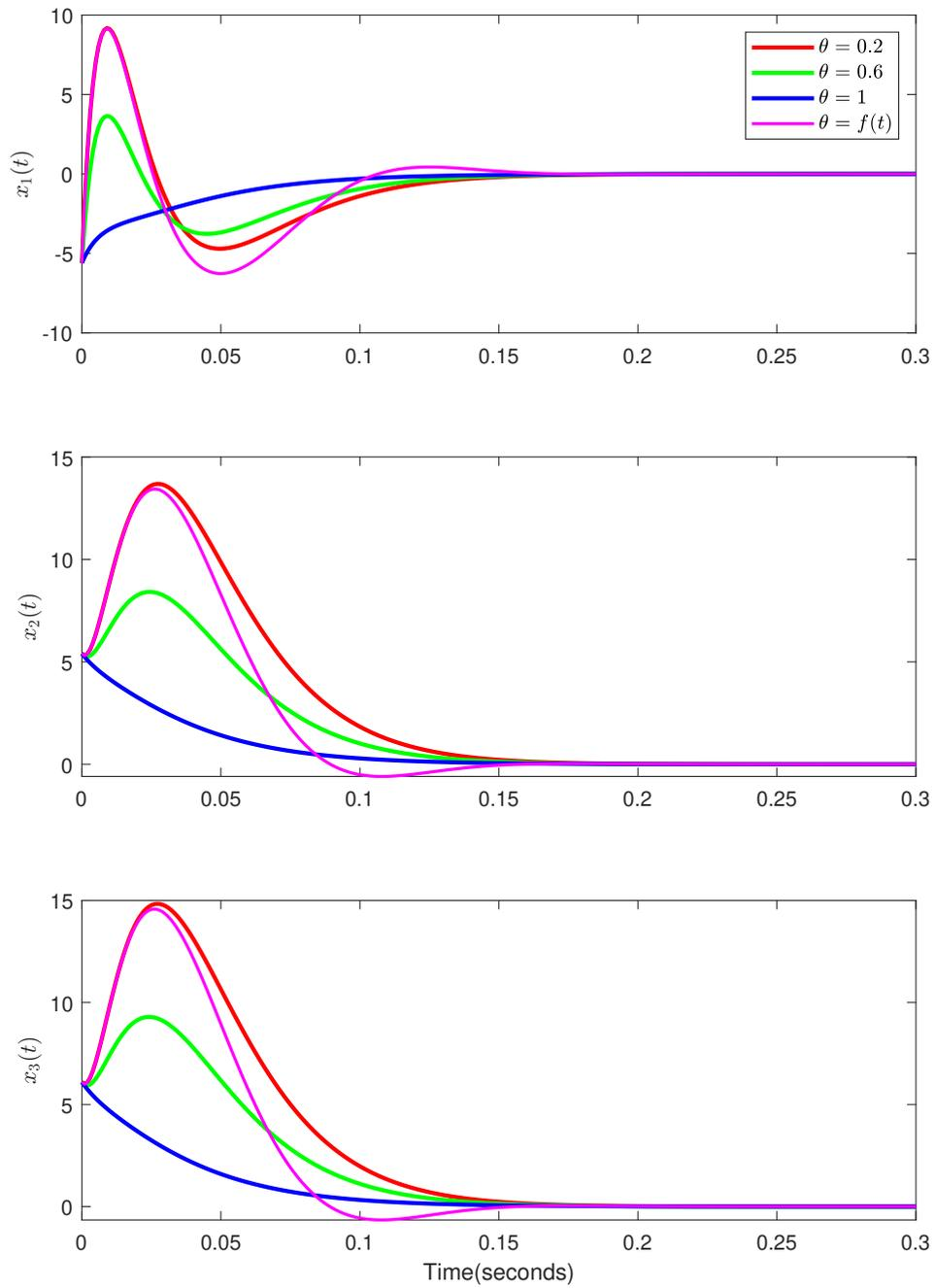
**Figure 7.** System response for different values/trajectories of  $\theta(t)$  using the shifting approach.
