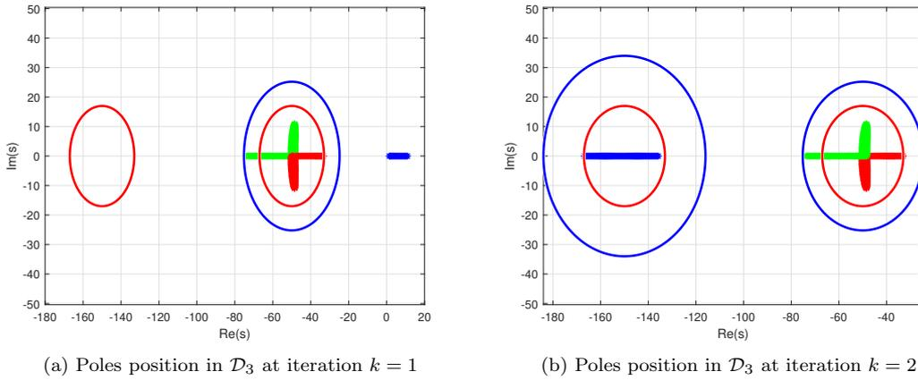
**Figure 5.** Position of the closed-loop frozen poles using the shifting pole clustering approach.
