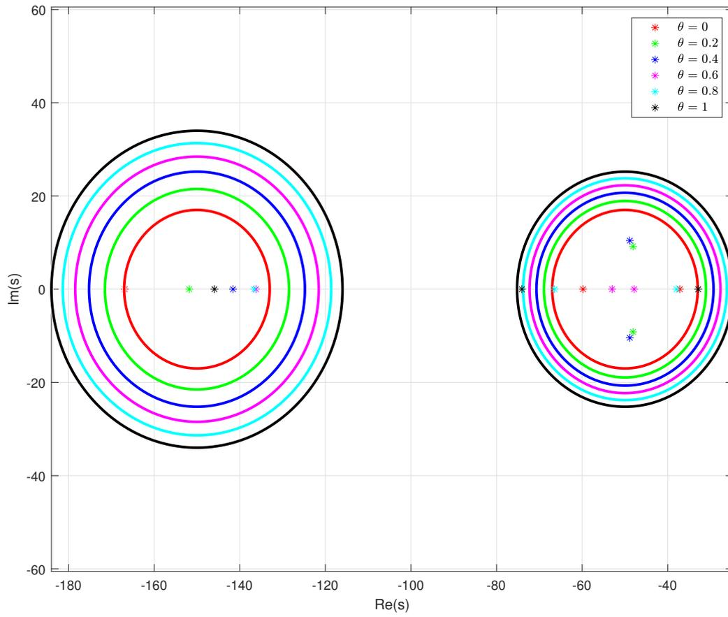
**Figure 6.** Position of the closed-loop poles for different values of  $\theta$  using the shifting approach.
