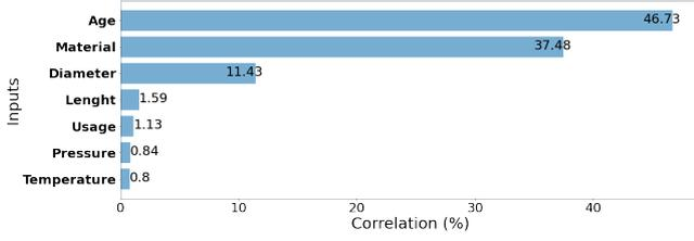
Fig. 1. Importance of different factors for failure rate.
