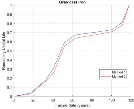
Fig. 2. RUL based on Weibull and CoxMLP.
