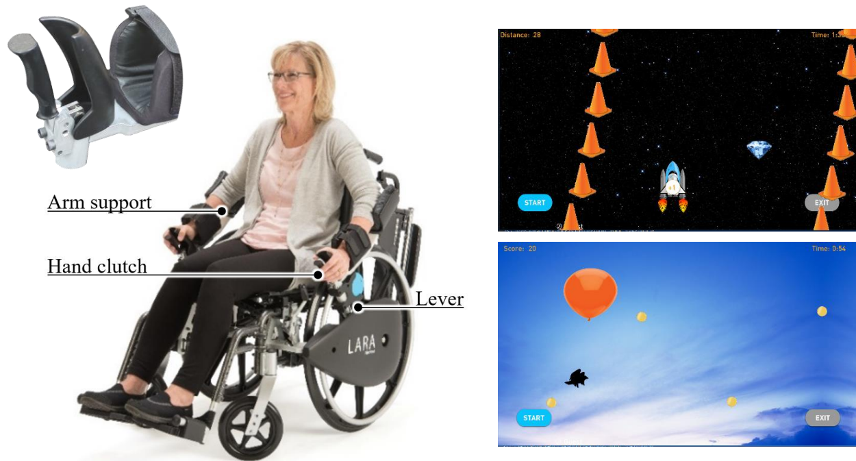
Figure 1. LARA is a novel lever drive wheelchair that has two modes of exercise: (1) playing a bimanual videogame (top right – the goal is to keep the spaceship between the cones by steering it by pumping the left and right levers) or unimanual videogame (bottom right – the goal is to raise and lower the balloon by pumping the paretic-arm lever faster or slower, to collect the gold coins) in a stationary mode using the instrumented levers as a joystick and (2) ambulating overground by bimanually propelling the wheelchair using the levers. The hand clutch (top left) is yoked to disk brakes on both wheels and activated during overground ambulation. It functions akin to a hand grasping the pushrim and provides maneuverability over level ground.
