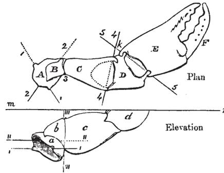
**Fig. 1** Willis’ drawing of the common crab’s claw used to explain how its joint axes are arranged (adapted from [2, p. 462]).
