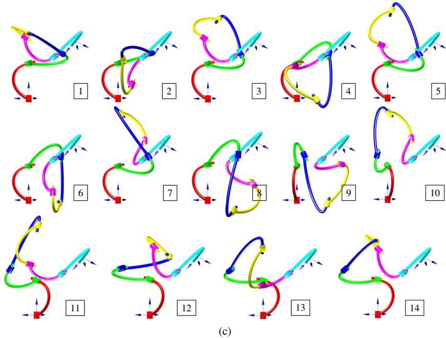
**Fig. 5** Using the method described in this paper, 14 real solutions are obtained for the inverse kinematics of the arm with the DH-parameters given in (a) and the end-effector located at Eq. (4). These solutions are numbered from 1 to 14 in (b), and the corresponding configurations are depicted to visually verify their correctness in (c).
