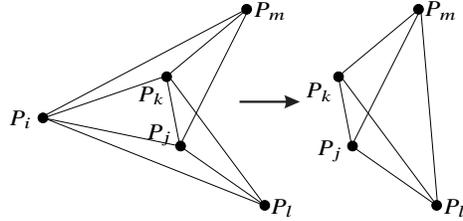
**Fig. 4** Substitution rule in a strip of tetrahedra that permits reducing by one the number of tetrahedra in the strip.
