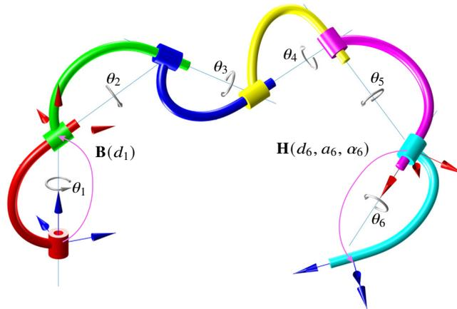
**Fig. 2** A generalized lobster’s arm, as defined by Duffy and Derby, is a 6R serial kinematic chain where all consecutive rotation axes intersect. In terms of standard DH-parameters, this means that  $a_i = 0$  for  $i = 1, \dots, 5$ .
