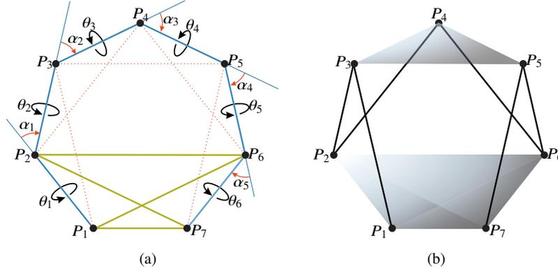
**Fig. 3** (a) Bar-and-joint framework associated with the generalized lobster's arm. The lengths of the bars in blue and dotted red are determined by the geometric parameters of the arm; and those in green, by the closure condition. (b) 4-3 Gough-Stewart platform whose associated bar-and-joint framework has the same topology as that of the generalized lobster's arm.
