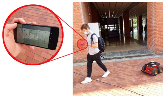
Fig. 11 Human-robot collaborative search example. The human is holding an smartphone through which he can communicate explicitly with the robot in a bidirectional manner. The robot can also keep track of the human movement while it can see him
