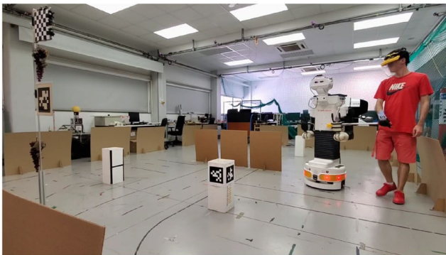
Fig. 8 Human-robot collaborative object transportation example. Human and robot transporting a bar. Force sensor attached to the robot's wrist with which it can the human's implicit intention and buttons on the handle of the object for explicit intention communication
