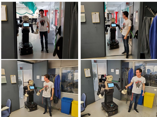
Fig. 9 Human-robot pair navigating through a narrow door. Top left : human-robot pair navigating side-by-side until they reach a door. Top right : human takes the lead but keeps taking into consideration the robot. Robot moves its left arm to allow the human to move forward. bottom left : human waits for the robot to finish passing through the door. Robot rolled up its right arm to reduce its footprint and moved its left arm to make the human to be in front of it. bottom right : human-robot pair recover their side-by-side configuration
