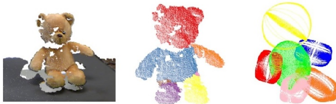
Figure 6: Level decomposition, replication and superquadric fitting on asymmetrical object [37]
