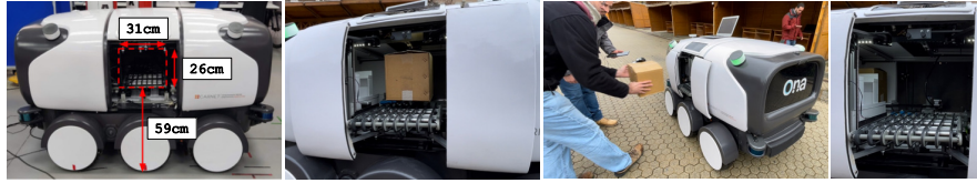
Fig. 2: Ona's storage management system with four internal compartments.
