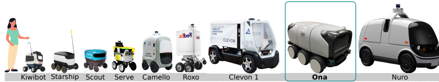
Fig. 1: Examples of last-mile delivery robots under development
