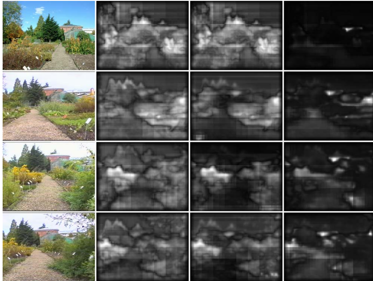
Figure 4 - Saliency maps computed for scene “B” for four different illumination conditions (one in each row). Note that there are slight changes in perspective between the images. Each source image (left column) was processed with lighting intensity normalization (second column), lighting intensity and illuminant color normalization (third column), and color ratios (fourth column). The whiter regions indicate the more salient parts detected.
