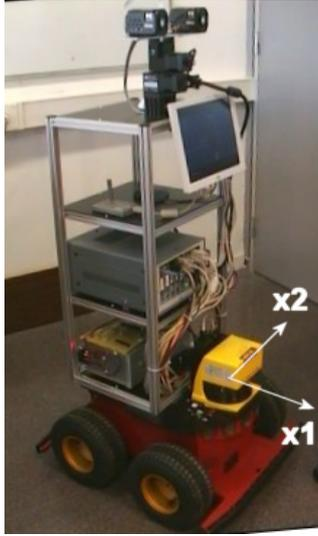
Fig. 1. The model for this nonlinear vehicle is used in the simulations, and is given in Appendix A. The Cartesian coordinates of the control point  $(x, y)$  are located on the projection center of the laser range scanner, and were purposefully chosen not coincident with the vehicle axle center.
