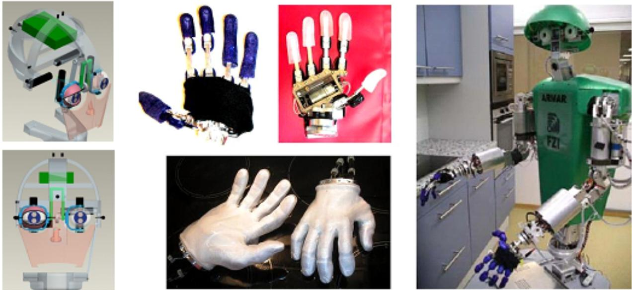
Fig. 1. Model of the proposed new robot head with two cameras for each eye (left), prototype of the five-finger FZK-hand (middle) and the humanoid robot ARMAR (right), Universität Karlsruhe.
