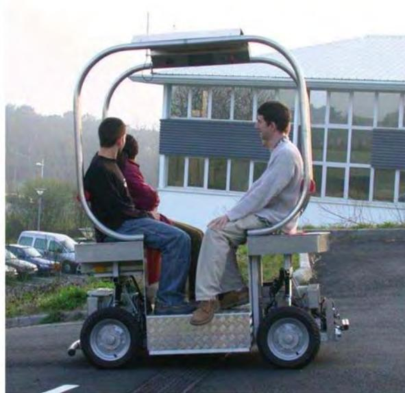
Fig. 9. Robucab mobile robot platform transporting four people.
