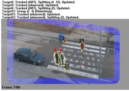
Figure 2: Trajectory acquisition from motion tracking
