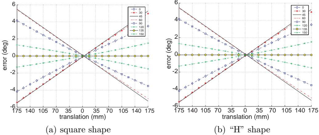
Figure 10. Error in the recovery of the epipolar direction for a fixed rotation of  $40^\circ$  about an axis inclined  $45^\circ$  on the target plane and an initial distance of  $5m$ , when lateral translations of the camera along the several directions listed in the insert are performed.
