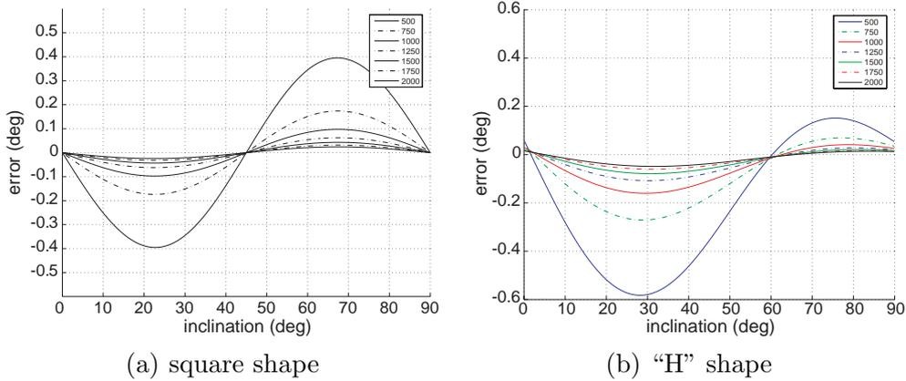
Figure 7. Error in the recovery of the epipolar direction when the distance from the camera to the target varies from 500 to 2000mm. The plot shows results for a camera rotation of  $40^\circ$  about an axis on the target with inclinations ranging from  $0^\circ$  to  $90^\circ$ .
