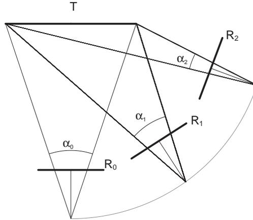
Figure 9. Starting with a frontoparallel target  $T$ , a first view  $\mathcal{R}_0$  is taken and then two other views  $\mathcal{R}_1$  and  $\mathcal{R}_2$  are taken;  $\mathcal{R}_2$  after a larger amount of rotation than  $\mathcal{R}_1$ . The maximum angle  $\alpha_i$  between the rays of the target projection decreases (and, thus, the projection becomes closer to a parallel projection) as the amount of rotation increases.
