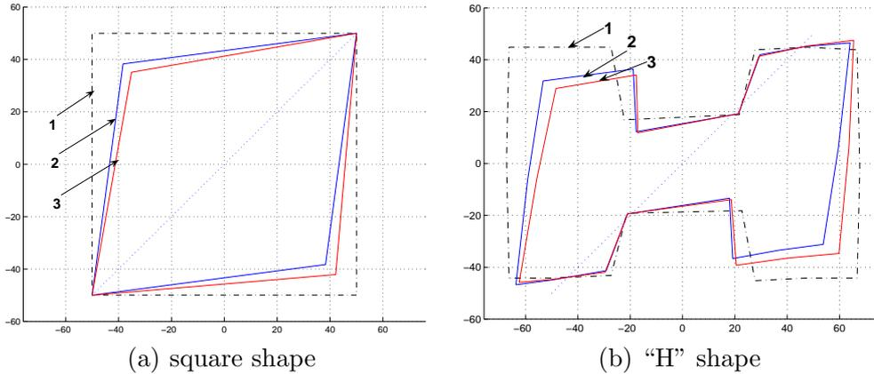
Figure 5. Difference in the projection of two control polygons for the two camera models discussed, after rotating the camera  $40^\circ$  about a  $45^\circ$  axis on the target, passing through the target center. 1) original contour, 2) weak-perspective projection, and 3) full-perspective projection.
