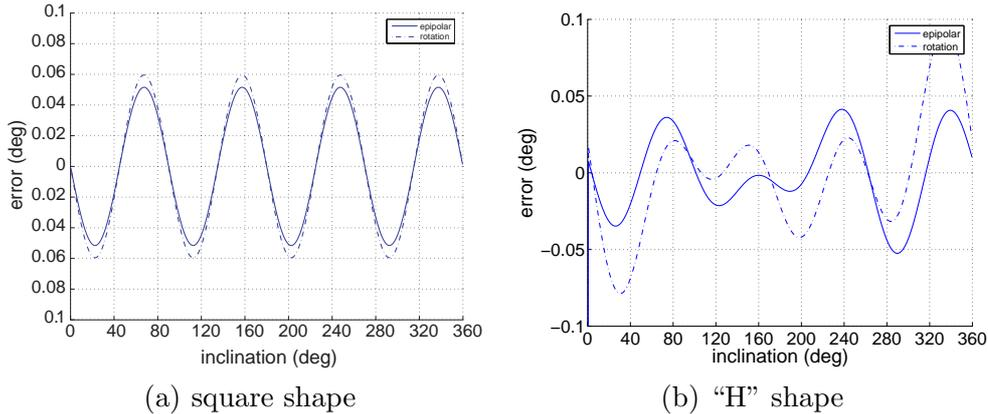
Figure 6. Error in the recovery after a camera rotation of  $40^\circ$  about an axis passing through the target centroid and whose orientation varies from  $0^\circ$  to  $360^\circ$ . The continuous line shows the error in the recovery of the epipolar direction, while the dotted one indicates the error in the recovery of the orientation of the rotation axis.
