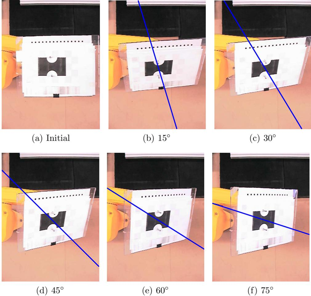
Figure 14. The first experiment with real images entails pairs of views consisting of the initial one plus each of the other five, corresponding to camera rotations of  $40^\circ$  about an axis on the target with inclinations sampled at intervals of  $15^\circ$ . The computed epipolar direction is displayed as a line passing through the target center.
