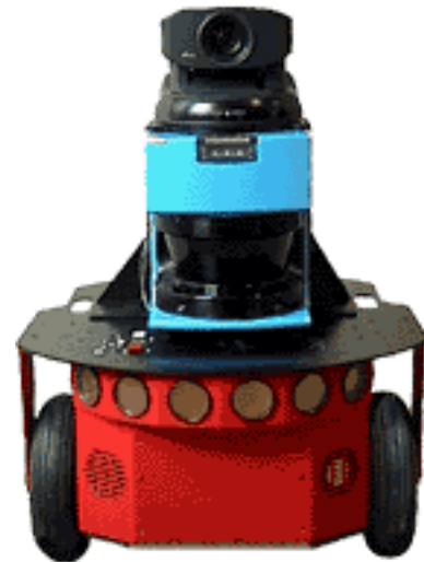
Figure 6. All ActivMedia robots may be configured with a variety of integrated accessories, including (DX shown here) a very high-performance laser range-finder and robotic pan-tilt-zoom color camera with onboard PC and framegrabber for color-tracking and surveillance.
