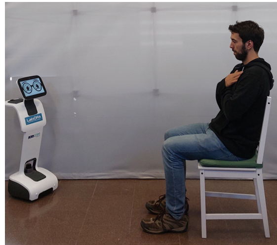
Fig. 1. Showcase of the frailty assessment. The robot monitors the patient (one of the authors) while he starts performing the TUG test.
