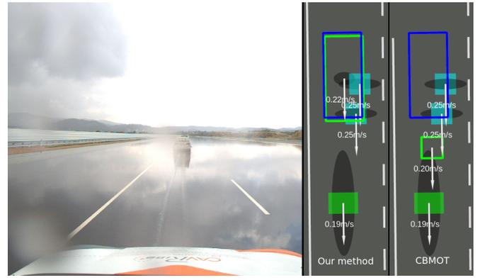
Fig. 5: **Traffic Jam Chauffeur scenario  $S_4$ : Image and detections.** We display information from the time  $t = 2.74$  s. On the left, the effect of the rain on the camera is visible. On the two right images, we see the detections of the camera (green square), and radar (cyan squares); along with the ground truth (blue rectangle) and the sensor fusion (green edges), our method in the middle and CBMOT [2] on the right.
