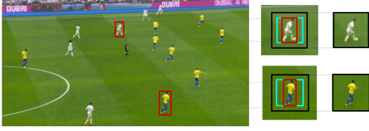
Figure 2: Video tubes extraction. Left: In every input image, a bounding box extraction (in red) per player is applied. Two instances are displayed in the figure. Middle: Zooming the selected player by means of a bounding box in red. To normalize data, the square that results from enlarging smallest rectangle side and the square after adding extra margin are displayed in cyan and black, respectively. Right: Final region to be cropped.
