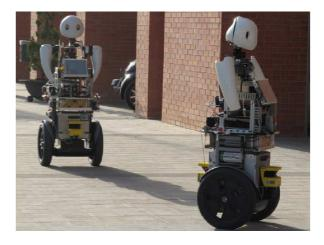
Fig. 1. Tibi and Dabo, urban service mobile robots.
