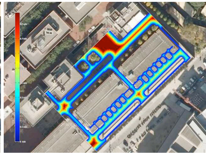
(b) Corresponding traversability map. Velocity varies from 0 m/s (blue) to 1 m/s (red).
