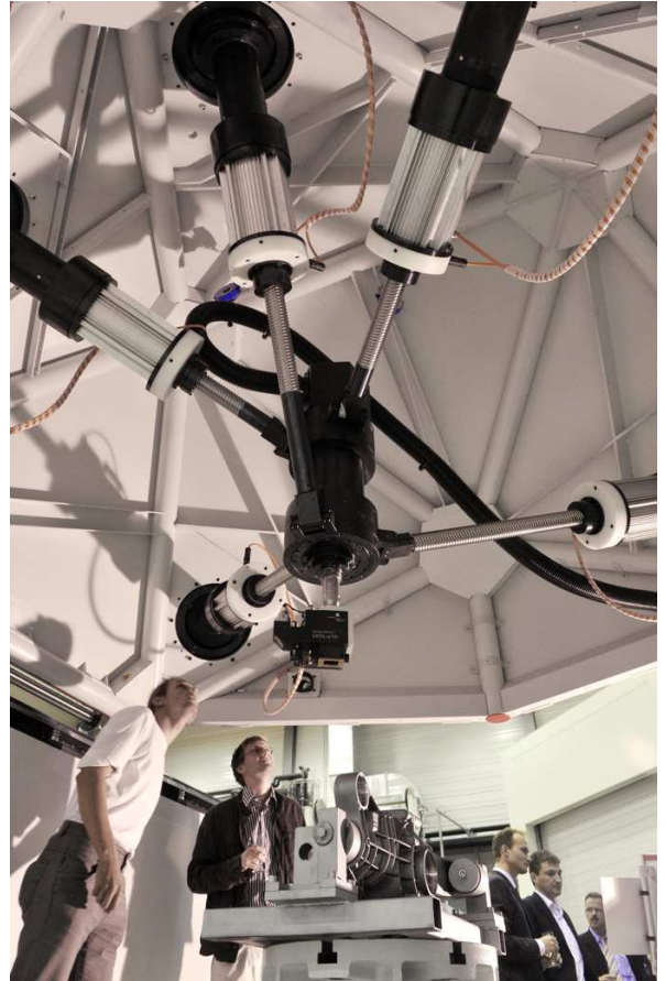
Fig. 1. A 5-axis milling machine, based on a pentapod, developed by Metrom Mechatronische Maschinen GmbH (reproduced with permission).
