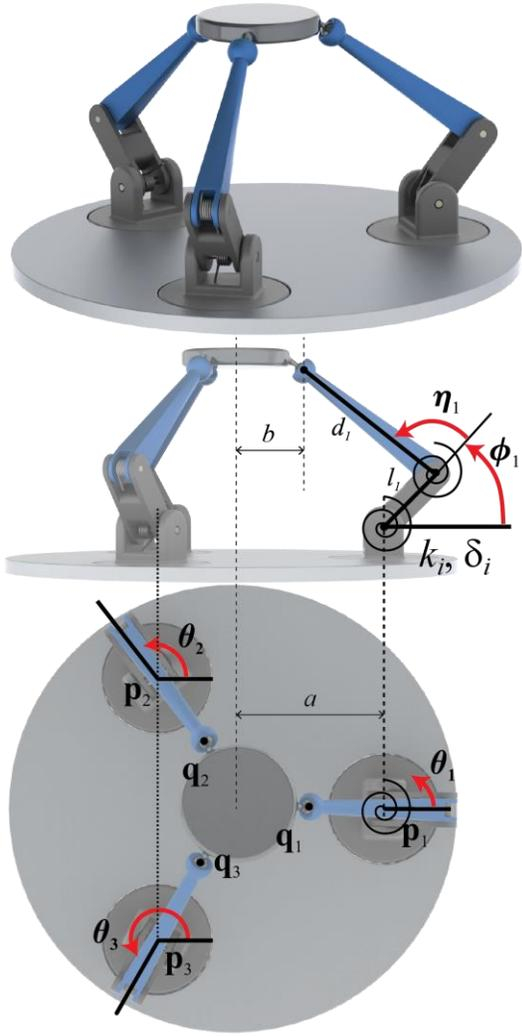
**Fig. 8 Notation for the 3-URS manipulator.**
