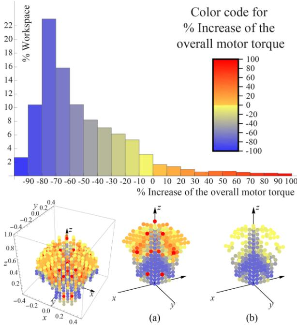
**Fig. 9 Top:** Histogram of the percentage of increase of the overall motor torque in each configuration of the workspace. **Bottom:** Each dot in the position workspace is colored depending on the mean reduction of the overall motor torque for all the orientations achievable from the dot position. From the left figure, (a) shows only a third to the figure, and (b) only the third and only configurations with reduction.
