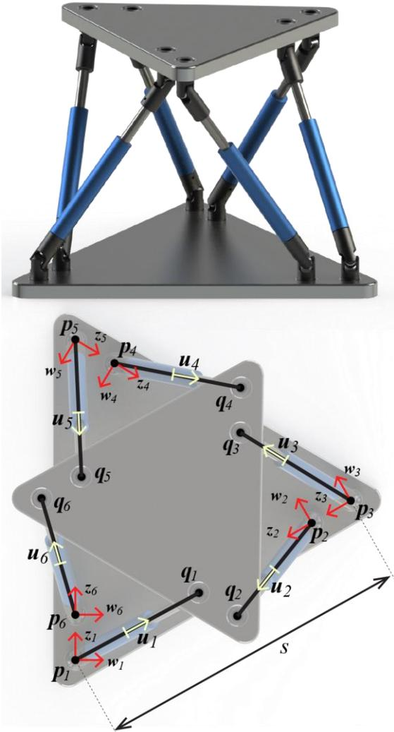
Fig. 3 Stewart-Gough platform equivalent to the octahedral design (top) and its corresponding notation (bottom). See Table I for coordinates of vectors  $z_i$  and  $w_i$ .
