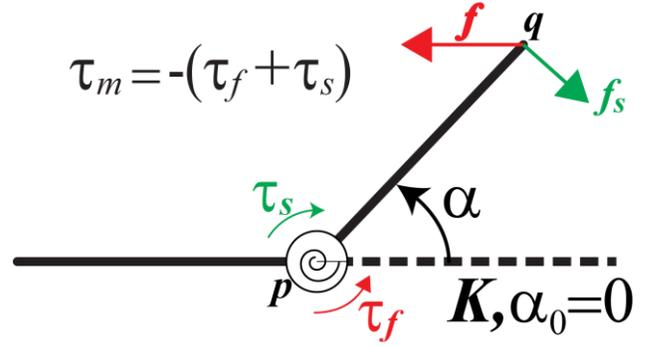
Fig. 2 Simple example of the combination of actuation torque exerted by the motor  $\tau_m$ , compliant torque exerted by the spring  $\tau_s$ , and reaction torque to the external force  $\tau_f$ .
