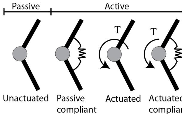
**Fig. 1** Classification of joints with and without compliance. In the parallel robot literature, any non-actuated joint is called passive, but as the passive compliant joint exerts a torque, we have to consider it as active for the static analysis.
