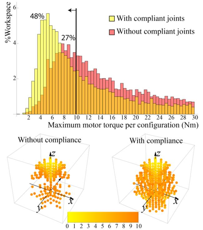
**Fig. 10 Top:** Comparison between histograms of the maximum torque values over the configurations of the workspace with and without compliant joints. **Bottom:** A representation of the static workspace. Each dot color represents the median torque for all the possible orientations in the corresponding position of the dot. All points where the maximum torque is bigger than 10Nm are discarded.
