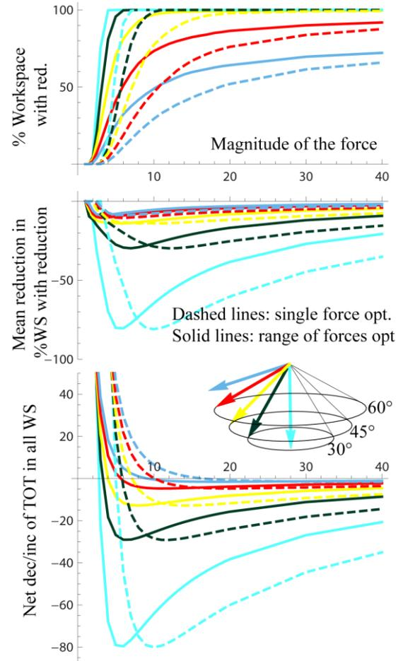
**Fig. 6 Percentages of reduction of the motor torque when changing the magnitude of the applied force. Each color corresponds to a different direction of applied force. Dashed (solid) lines are results of a manipulator using the compliant parameters in equation (30) (equation (31)).**
