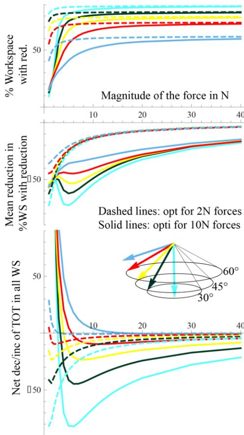
**Fig. 11 Comparison of manipulators using the compliant parameters optimized for a range of forces of magnitude 10N (equation (36)) and for a range of forces of magnitude 2N.**
