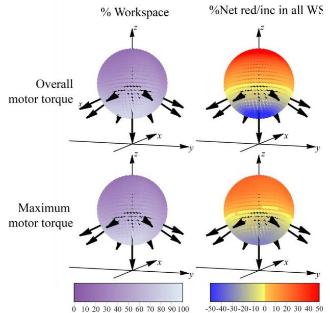
**Fig. 12 Similarly to Fig. 7, each dot represents a direction of the external applied force, and its color the percentage of workspace with reduction (first column) and the net reduction (second column). Reductions of the overall torque are shown in the first row, while reductions of the maximum torque in each configuration are shown in the second row.**
