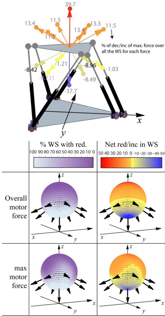
**Fig. 7 Top:** Each applied force is associated with a dot in a sphere. **Bottom:** The colors represent the percentage of the workspace with reduction (first column) or the net increase (second column) of the overall torque in the first row, or the maximum motor torque in the second row.
