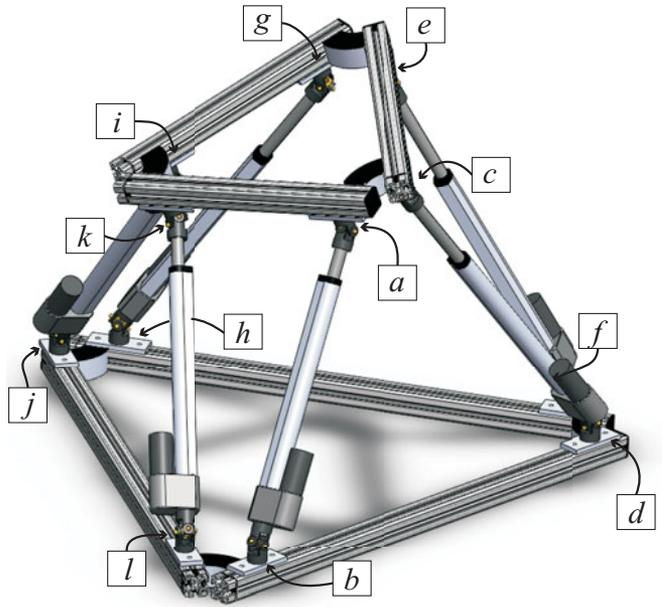
Fig. 1. The 6-6 Stewart platform and adopted labeling for its leg attachments.
