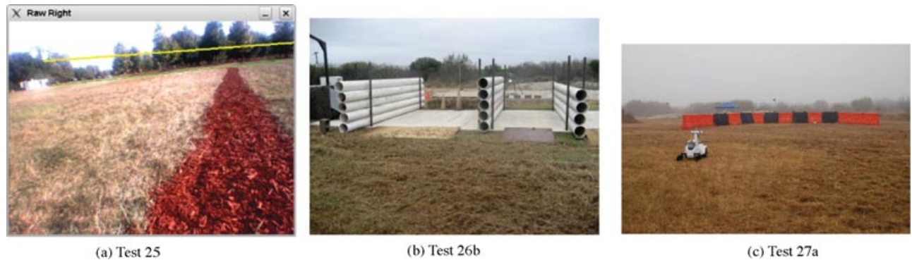
Figure 18. Views of three final tests. In (a), a robot's-eye view of the beginning of Test 25. The copse in the distance could be avoided on the right or left. The yellow line is the robot's horizon from a noisy INS, and the green line is the VO-stabilized horizon. In (b), a pipe corridor from Test 26b: note the blocked left corridor. In (c), Test 27a shows the Jersey barrier, with the goal immediately behind.
