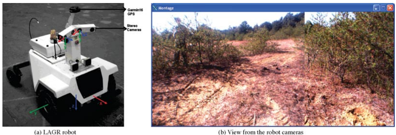
Figure 1. (a) LAGR robot with two stereo sensors. (b) Typical outdoor scene as a montage from the left cameras of the two stereo devices.
