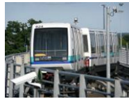
VAL 208 in 2000 with PM in-wheel motors
