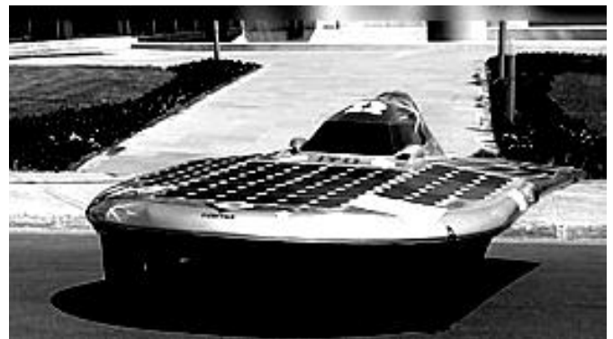
Fig. 1. Students' project - experimental solar + accumulator car.
