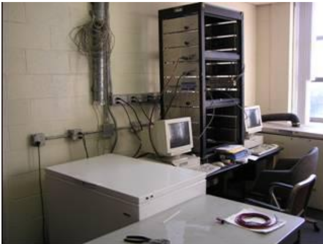
Fig. 2. Battery Exerciser at the Battery Evaluation Lab at UMass Lowell. The central tower houses two sets of eight current regulators and their analog/digital multiplexers. One of the environmental chambers is in the foreground.
