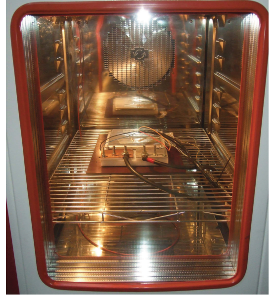
Fig. 14. Climate chamber to guarantee a constant temperature of 40^\circ\text{C} during cycling.
