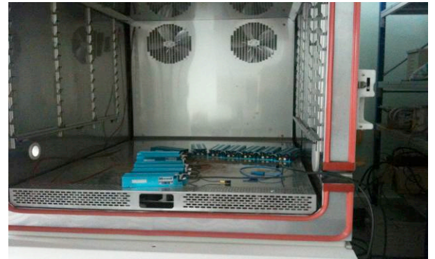
Fig. 11b Test of UC complete pack the climatic room at FEMTO-ST Institute
