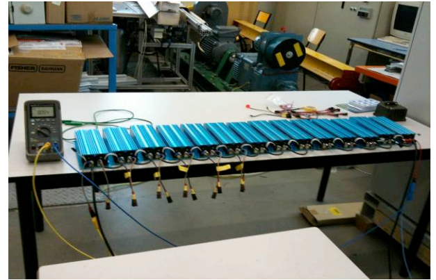
Fig. 11a Photography of the UC complete pack designed for 'PHEBUS' vehicle
