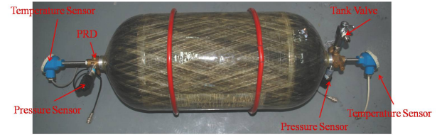
Figure 4. The Hydrogen Tank
