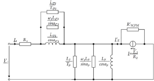
Figure 4 Extended equivalent circuit for permanent magnet synchronous machines considering iron losses
