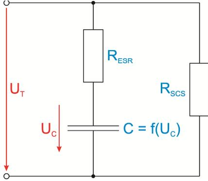
Figure 1 Equivalent circuit of a double-layer capacitor cell
