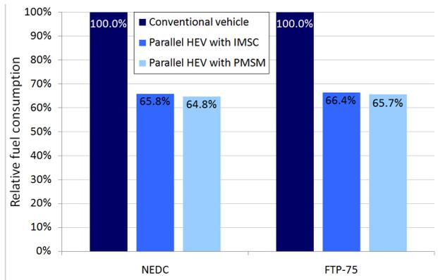
Figure 10 Relative fuel consumption of a hybrid electric vehicle during New European Driving Cycle and FTP-75 Driving Cycle
