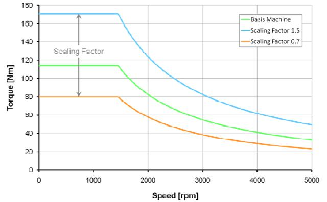
Figure 5 Influence of axial machine scaling on mechanical operating area depending on the axial scaling factor  $k_a$
