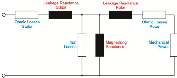
Figure 2 Equivalent circuit of an asynchronous induction machine
