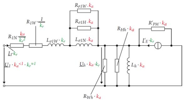
Figure 7 Scalable PMSM equivalent circuit
