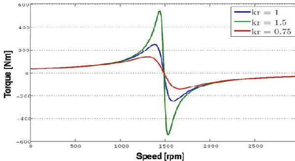
Figure 8 Influence of radial machine scaling on the IMSC's speed-torque-characteristics depending on scaling factor  $k_r$ .
