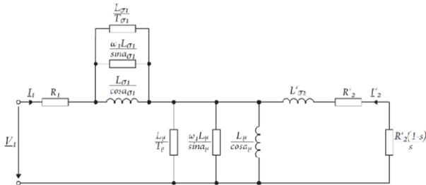
Figure 3 Extended equivalent circuit for asynchronous induction machines with squirrel cage considering iron losses
