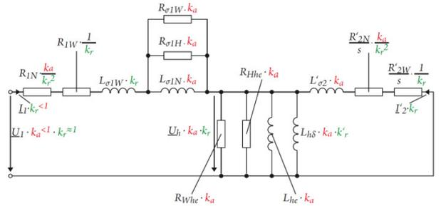
Figure 6 Scalable IMSC equivalent circuit
