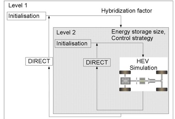
Figure 9 Schematic structure of the applied two-level optimization procedure
