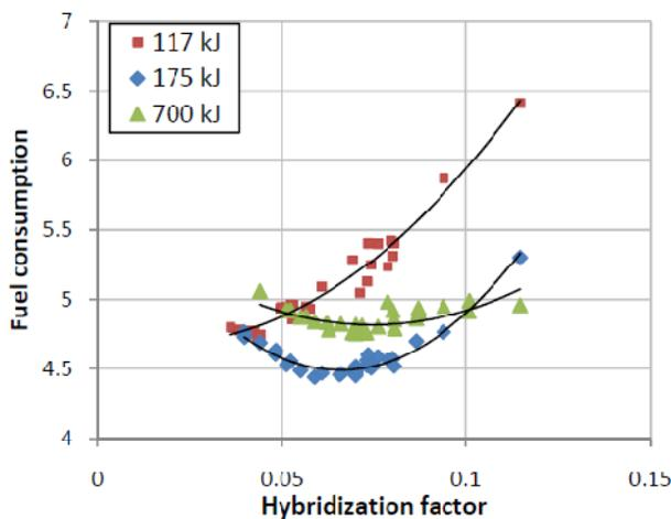
Figure 11 Influence of hybridization factor and energy storage size on fuel consumption (Middle class car, New European Drive Cycle)
