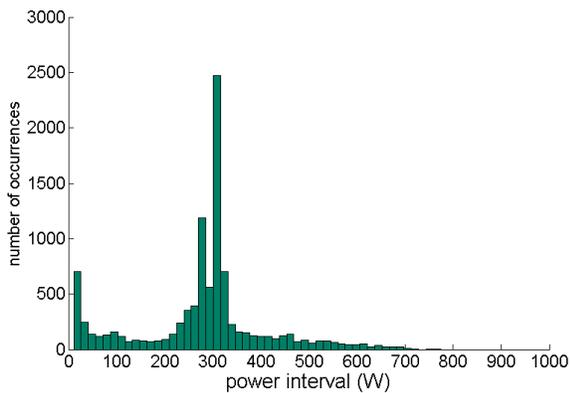
Fig. 7. Histogram of power spectrum of  $P_{bat}$ , when using controller number 2
