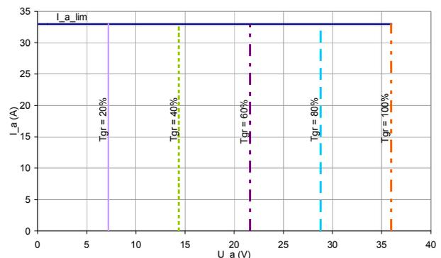
Fig. 2. Controller output characteristics when turning the pedals.
