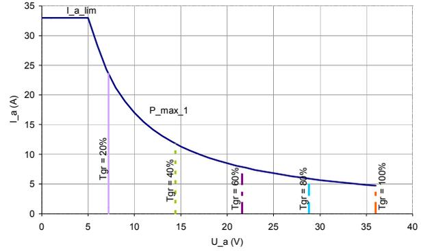
Fig. 3. Controller output characteristics when turning the pedals.
