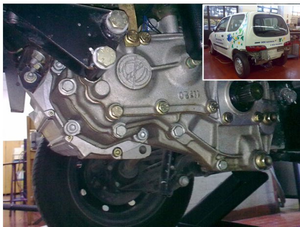
Fig. 1. Photography of the induction motor and of the “Fiat Seicento Elletra”.
