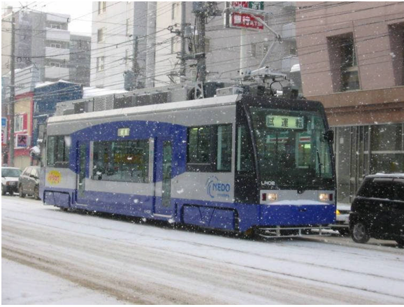
Fig. 5. Contact-wire/battery hybrid LRV 'Hi-tram'.
