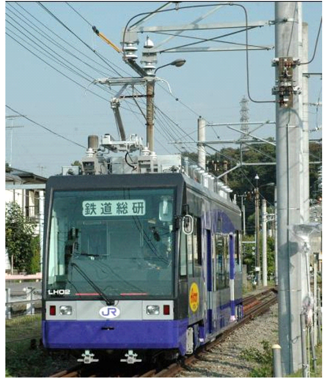
Fig. 7. Quick charging from rigid contact wires.
