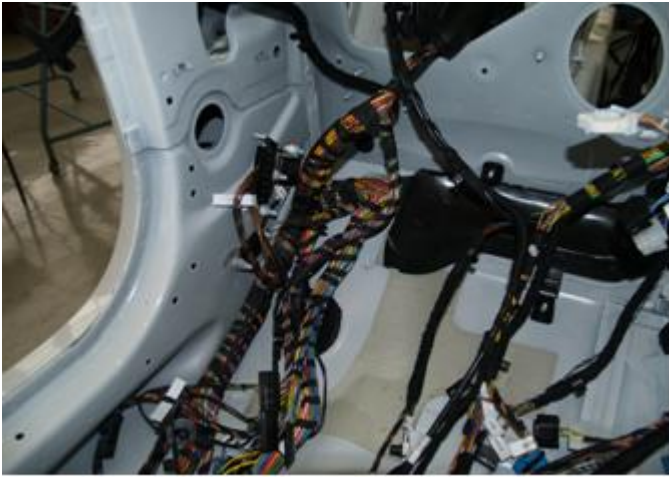
Figure 3. Detail of the wiring harness (driver floor) with wires of communication busses and the power supply as well as some grounding bolts on the car body.
