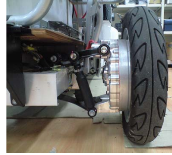
Fig. 10. In-wheel motor (Direct drive motor).
