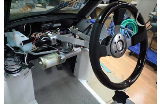
Fig. 11. Driver-friendly reactive torque motor.
