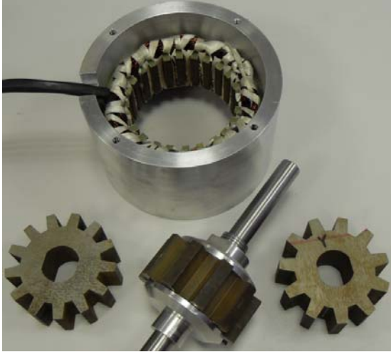
Fig. 15. 12/10, 12/11, and 12/13 stator/rotor pole FS prototype machines.
