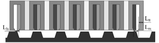
Fig.15 Optimization variables for minimum cogging force.
