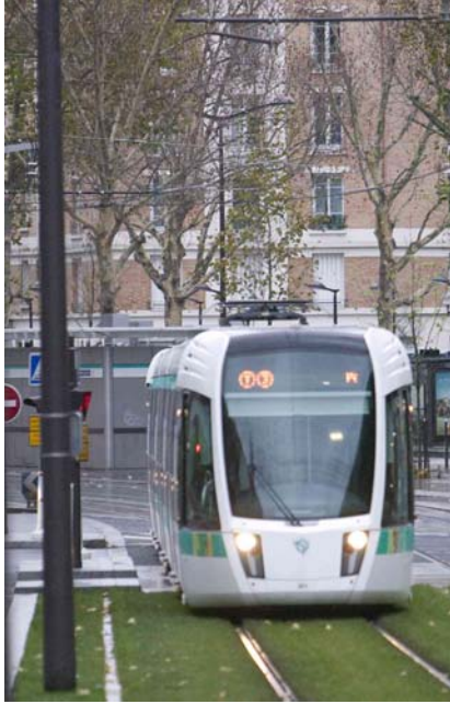
Figure 6. Train 301 running pantograph lowered
