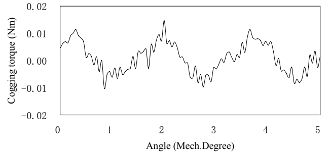
Fig. 13. Cogging torque waveform.
