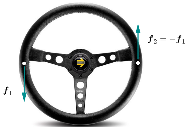
Figure 2.10: Couple of forces acting on a steering wheel.
