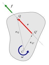
**Slide 13** As in the case of a particle, P measures the kinetic energy transmitted by the force to the body. The example shows different situations where P is positive, negative, or zero.
