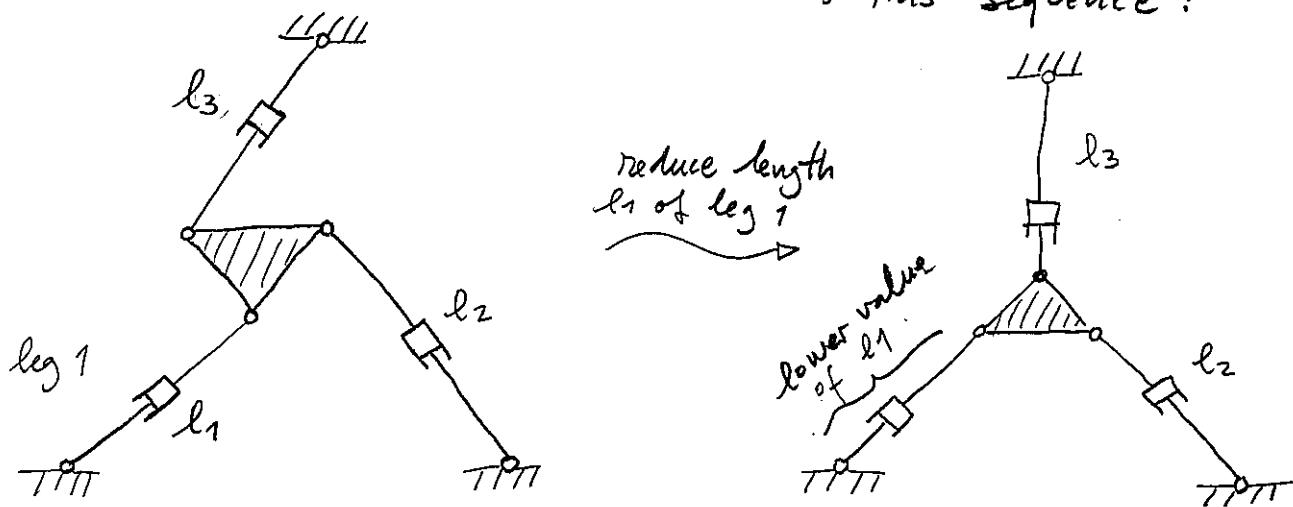
Initially, with actuators locked  $\rightarrow$  mechanism is rigid, Leg 1 is unlocked then, and its length is reduced to bring the robot to a singularity
