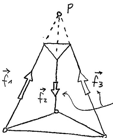
The concurrence of the three leg lines on  $P$  allows the existence of such self-stresses.
