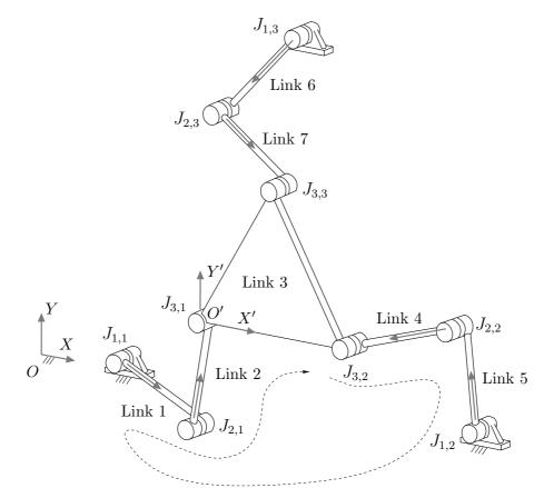
In frame OXY, the loop-closure equation of the indicated loop is:
