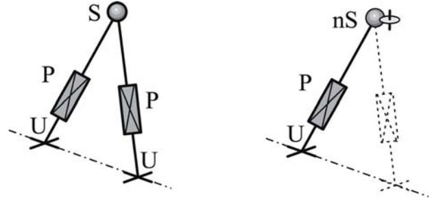
Figure 3. UPnS limb (right) generated by substituting an nS pair for the S pair in the two UPS limbs with coalesced S pairs (left).
