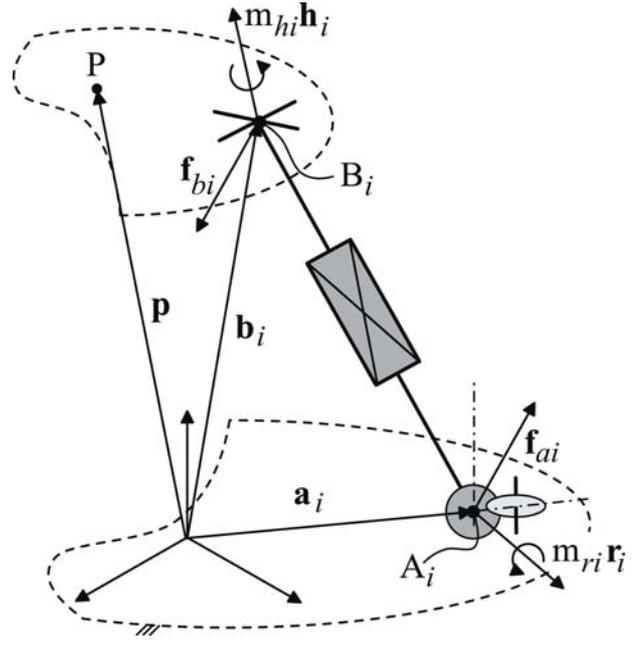
Figure 6.  $i^{\text{th}}$  limb of type nSPU: free-body diagram.
