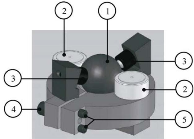
**Figure 1.** 3D CAD model of one out of many different manufacturing schemes for the nS pair: (1) sphere, (2) roller (carried out through a roller bearing), (3) spherical bearing [there are three spherical bearing (only two are visible) that forbids the translation of the sphere], (4) pre-load adjust screw, and (5) parallelism adjust screws.
