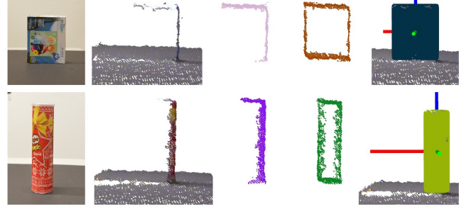
Fig. 3. The complete mirroring pipeline. From top to bottom, the mirroring process with a box and a cylinder object (The capturing device can be assumed at the right side of the image): a) RGB side view of the object, b) captured point cloud of the scene, c) segmented point cloud of the object, d) mirrored point cloud with the segmented cloud, e) SQ representation of the object.
