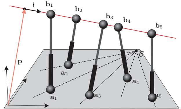
Fig. 1. A 5-DoF 5-SPU parallel manipulator with collinear attachments in the platform and coplanar in the base.
