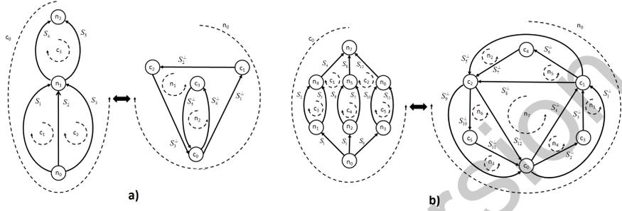
**Fig. 3** Graph representation of a) a hybrid mechanism and b) a Delta mechanism and their corresponding dual mechanisms. In both cases, the mobility of the dual mechanism corresponds to the overconstraints of the original mechanism and vice versa.
