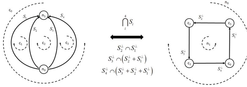
**Fig. 2** Graph representation of a parallel mechanism with four legs and its dual single closed-loop. The screw system over the big arrow represents the mobility of the parallel mechanism and the overconstraints of the single closed-loop. The screw systems below the arrow represent the overconstraints of the parallel mechanism and the mobility of the single closed-loop.
