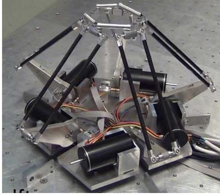
**Fig. 1** The 5 DOF PentaG robot with configurable platform. The configurable platform can translate in 3 directions and has 2 internal DOF, providing additional rotation and grasping capabilities. This architecture was used to develop both a haptic device and a pick-and-place robot.
