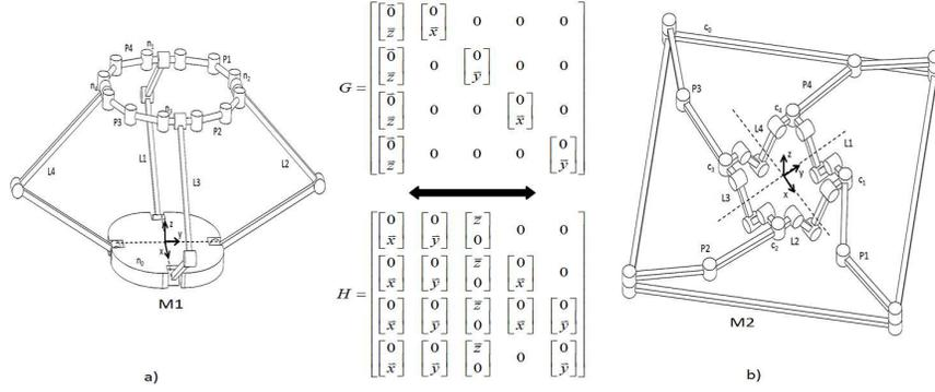
**Fig. 5** Dual mobility and overconstraints of two PMCPs.  $G_L$  represents the mobility of M1 and the overconstraints of M2.  $H_p$  represents the mobility of M2 and the overconstraints of M1. Each line of a matrix of mobility uses twist screws to represent the mobility of a leg end-effector  $n_i$  or  $c_i$  relatively to the base. Each line of a matrix of overconstraints uses wrench screws to represent the internal stresses in a platform limb between two end-effectors.
